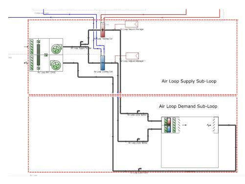
Notice that the hot/cold ducts (together with coils) are represented more or less as direct equivalents, whereas all the other loop components (including the mixed air system manager) are combined within a single AHU component.
