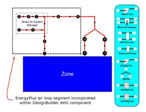
For clarity and to provide a more familiar layout to designers, the various EnergyPlus air loop supply components which constitute the air handling section of the loop are incorporated within a bespoke
