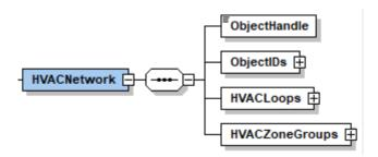
An EnergyPlus HVAC network consists of various components that are connected physically in the actual system by ducts, piping, etc. Every component in the network has an inlet and outlet "node". In the actual system, a node might be a point in the system at which fluid properties can be measured. In an EnergyPlus simulation, the nodes are points at which fluid properties are evaluated
