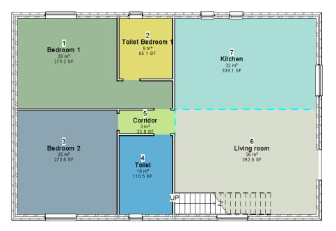
You can use the <u>Room Separation Lines</u> tool to add and adjust room boundaries. They are useful for designating one room within another when there aren't walls. In the sample above Room separation lines are room-bounding between the kitchen, living room and corridor zones.
